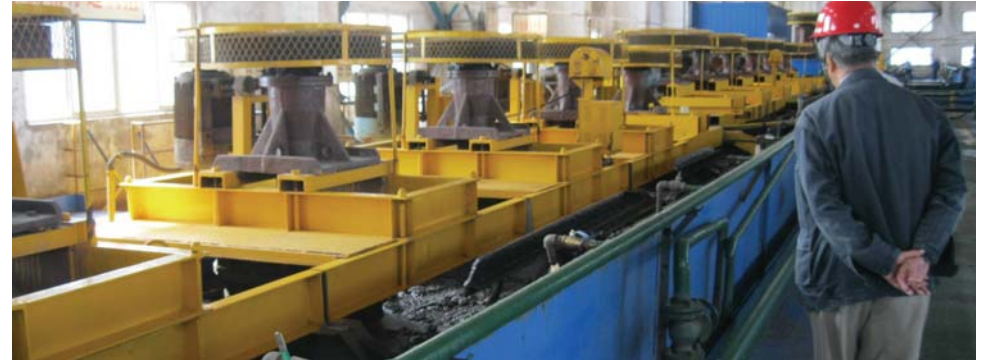
赤铁矿反浮选 Hematite by Reverse Flotation Separation
