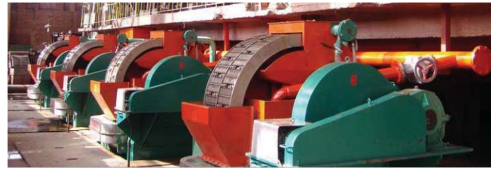
赤铁矿强磁选 Hematite by Strong Magnetic Separation
