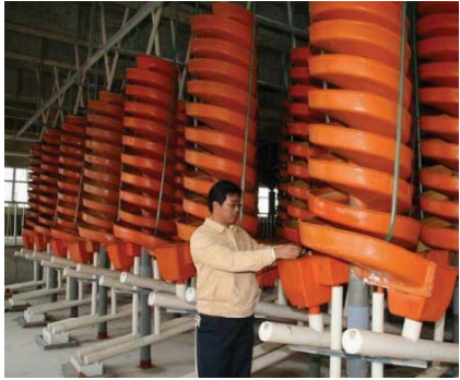
铬矿重选 Chromite by Gravity Separation
