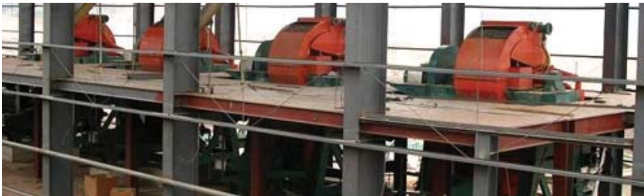
铬矿强磁选 Chromite by Strong magnetic separation
