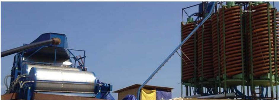
赤铁矿重选 Hematite by Gravity Separation
