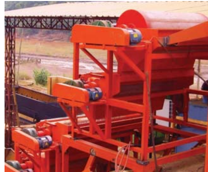
铬矿重选 Chromite by Gravity Separation
