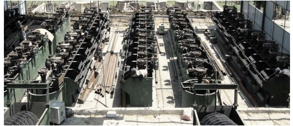
萤石矿浮选 Fluorite Flotation Separation
